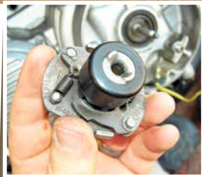
Replacing the old ignition with electronic
